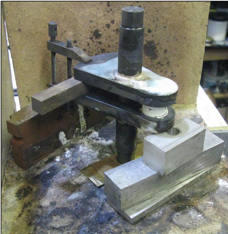
In case you wondered, the white stuff on the crank pin is Tipex. It is a good medium to use to stop solder flowing and it also protects the surface from heavy oxidation when using a lot of heat. I should have put some on the axle bearing areas as well but forgot! Yes I know there are machine marks ..... the webs were cut on
