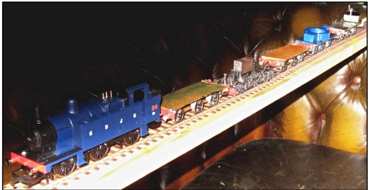
tender chassis's from Sutherland Models. A hefty white metal casting which needed a good deal of cleaning and filing. The rotor (blue) was a piece of steel in a jar. The brake wagon was a metal cube, drilled for the brake rod and a Kays wheel and crankpin complete the set. The wagon flats were a mixture of heavy duty plastic card and some thin springy steel.
